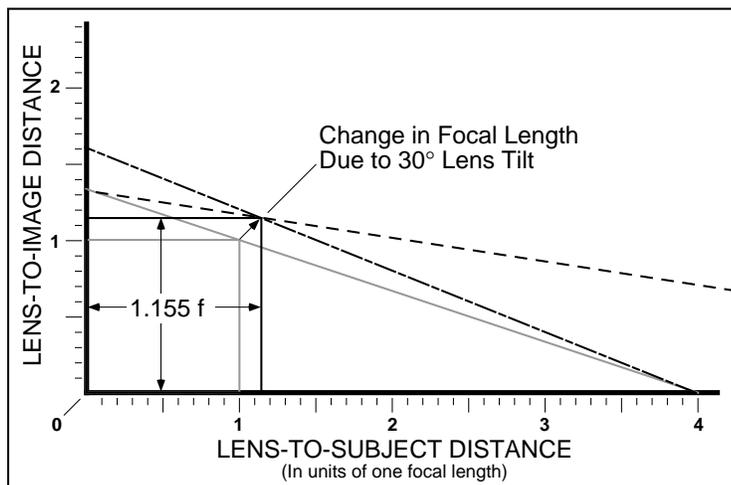
Figure 4: For a lens tilted by  $30^\circ$ , the focal length is effectively increased by 15.5%. If the lens-to-object distance remains unchanged, the image distance must be increased as shown by the dash-dot line. Otherwise, the camera is focused beyond the object, as shown by the dashed line.
